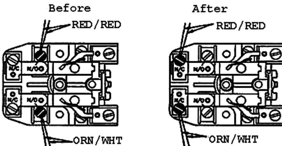
N.O. - Normally open contact    N.C. - Normally closed contact
